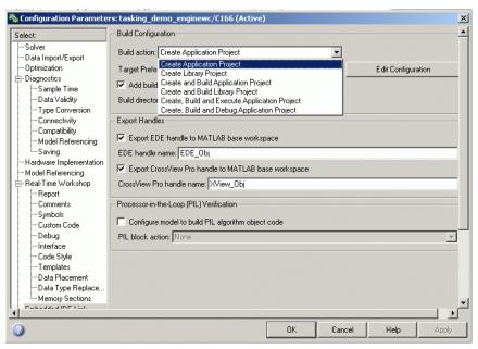
Using this drop-down list, you can set what action to take after the Real-Time Workshop build process completes. You can create application and library projects in the TASKING EDE and then stop, or you can also choose to build, execute, or debug.
